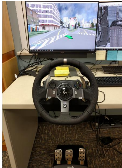
Figure 9. Logitech driving simulator setup with pedals (left panel). Participants were only required to use the steering wheel and the gas pedal to drive through the virtual city.
